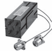
Built-in duplexer (left) Built-in RF pre-selector (right).
